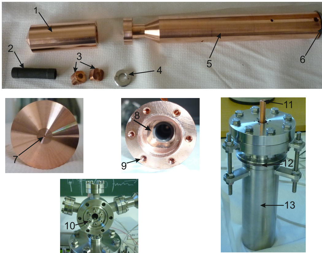
Figure 3.6: This figure shows the cold finger parts before they are assembled. (1) is the core of cold finger, (2) is the graphite tube which is inserted inside cold finger as seen in (8). (3) the mounts holding a BK7 window between them at Brewster's angle, which are themselves clamped down by a threaded ring (4). (5) is an other copper tube connected to the cold finger via (9) to extend the cold finger to reach a view port of the vacuum chamber. (6) is a steel mount, which connects the entire cold finger to an external view port seen in (10). (11) shows the physical contact between the cold finger and an LN2 tank via a copper rod. The flexible tube (3) is used to suppress any stress or expansion on the contact point (11) during the cooling. (13) is the LN2 tank.
