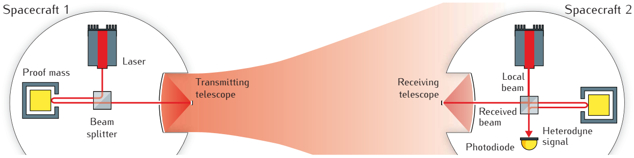
Figure 2.2: One laser link between two spacecraft of a gravitational wave observatory. A remote laser (on Spacecraft 1) is transmitted to Spacecraft 2. Here it gets interfered with a local laser of a different frequency and the heterodyne signal is detected. Gravitational waves alter the proper distance between the spacecraft resulting in a phase shift of the signal. Freely floating proof masses form the end points of the inter-spacecraft interferometer arm to suppress the influence of spacecraft position jitter on the actual arm length. To construct a complete observatory arm, one also needs the reverse link.
