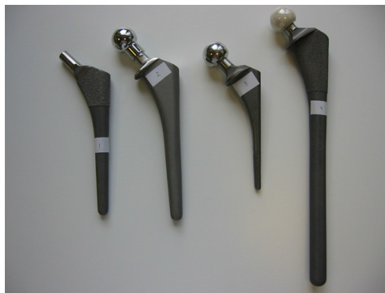
Fig. 17: Photographs of different hip prostheses made of titanium alloy (nr. 1, 3 and 4) and Co-Cr-Mo alloy (nr. 2). The prostheses are equipped with heads made of stainless steel (nr. 2 and 3) and of ceramic material (nr. 4) (from ref. [12]).
