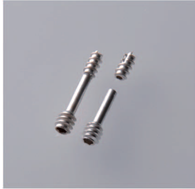
Fig. 3: A biodegradable orthopedic MgYREZr screw, length is 6 mm (from ref. [52]).
