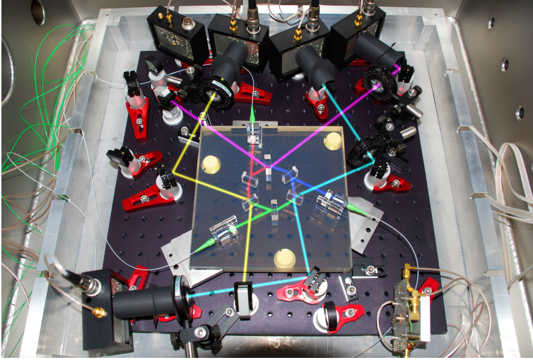
Figure 3.19: Picture of the hexagonal interferometer testbed. Three heterodyne beat-notes with a zero phase combination are generated on the bench, corresponding to the violet, light blue and yellow beams. The optical signals are detected by the photoreceivers, and their phases are extracted by the phasemeter to get an estimate of the full chain performance. The three-signal combination can reveal non-linearities. Once performance is achieved using mW signals, optical powers in the pW range can be used to test the noise contribution of the photoreceiver. Credit: Daniel Penkert.
