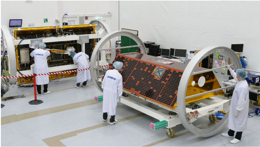
Figure 1.3: The two GRACE-FO satellites in a clean room at the iABG facilities in Munich, Germany. The assembly of the final components finished in the second half of 2017. In 2016 and 2017, a series of tests at spacecraft level verified all requirements prior to launch. This included environmental and functionality tests. Image credit: Airbus DS GmbH, Mathias Pikelj.
