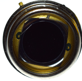
Figure 3.14: Picture of one of the two PC50-7 samples tested in STELA. The PC50-7 is a silicon photodiode frequently used in experiments at the AEL.
