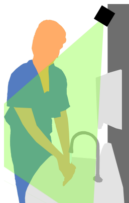
Figure 2. Illustration of the setup in practice, with a time-of-flight sensor facing downwards observing the scene around a disinfection dispenser.
