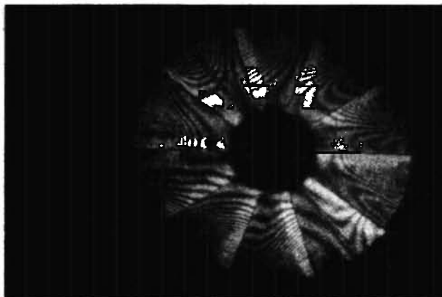
Fig. 19: Interferogram of the impeller at n = 11900 rpm.
