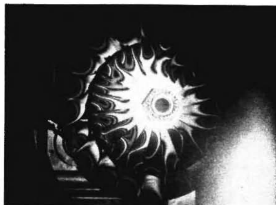
Fig. 6: Holographic interferogram of the radial impeller at rest excited to vibration in a laboratory test. f = 5500 Hz.
