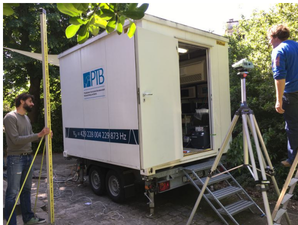
Figure 4.14: On the left: the spirit leveling measurement performed by geodesists of the Institut National de l'Information Géographique et Forestière (IGN). On the right: a map showing the position of the transportable clock in respect to marker 200 and a picture of the vacuum chamber highlighting the reference point (point 4) chosen on the top of the Zeeman slower window.
