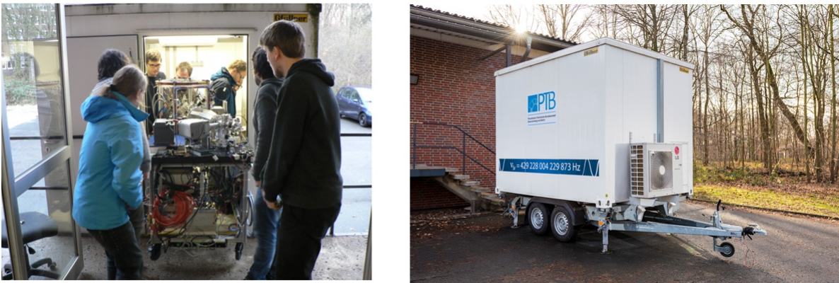
Figure 3.6: After initial tests in the laboratory, we moved the optical clock components inside a car trailer (left). A view of the car trailer from the outside is showed in the figure on the right. It can be pulled by a van and has an air conditioning system.
