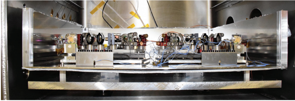
Figure 4. Layout (a) and photograph (b) of the experimental set-up of a free beam connection between two co-rotating benches. Off-the-shelf components and adjustable mounts are used on a carbon breadboard, placed on two aluminum plates sitting on two rotary tables. (a) 2D sketch of the free beam link including beam rays simulated with IfoCAD. (b) Photograph of the free beam link in the vacuum chamber inside the thermal shielding.
