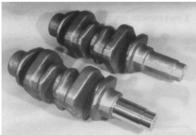
Fig. 3 Crankshaft before and after turning operations
