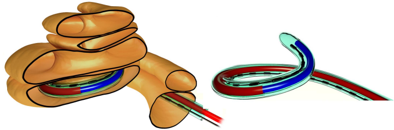
Figure 1: Envisioned steerable electrode array with a helical tube (red) and wire (blue) in a guide channel for insertion into the scala tympani (lower duct of cochlea).
