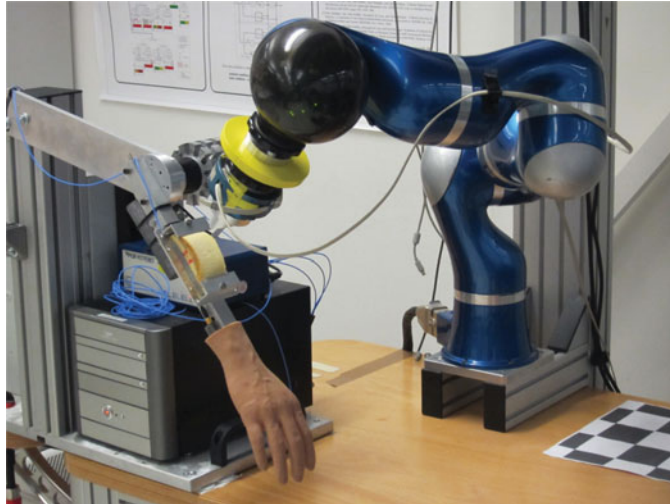
Fig. 7 Collision setup for LWR-III/PMLA experiments.
