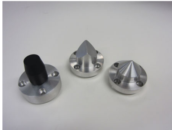
Fig. 9 Differently shaped industrially relevant robot end-effectors for plane, line, and point impact.
