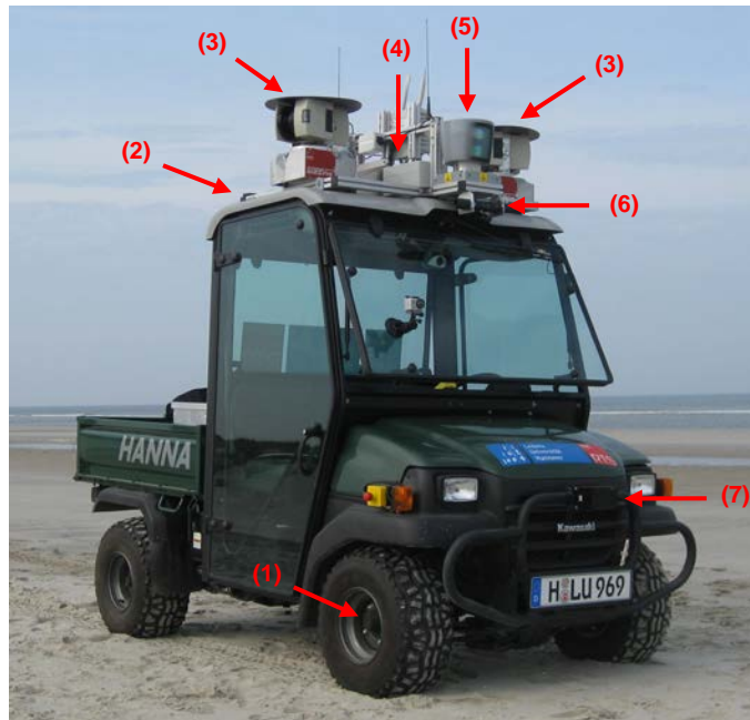
Figure 1. Autonomous robot RTS-Hanna: (1) wheel odometry, (2) D-GPS Trimble AgGps 114, (3) ScanDrive, (4) Gyro PerformTech Gu3024, (5) Velodyne HDL-64E, (6) Microsoft Kinect, and (7) ibeo LUX.
