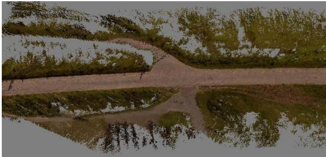
Figure 5. Coloured 3D scans merged by D-GPS position, viewed from the top, with parts invisible to the scanner displayed in Grey.
