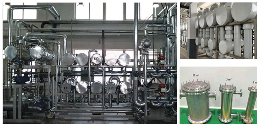
Fig. 9 Apparatus for dehydration of ethanol (1500 tons per year), left, apparatus for dehydration of acetonitrile (15 000 tons per year), right above, and membrane modules for dehydration, right below, at Jiangsu Nine Heaven High-Tech Co. Ltd (from ref. 243).
