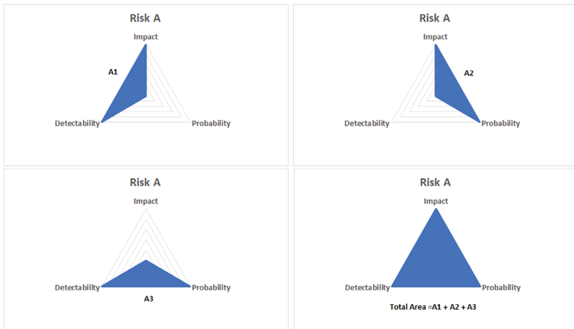
Figure 2. The area under the radar chart. This figure shows the total area of the radar chart. Each area of the subtriangles is calculated based on the conventional formula.
