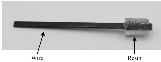
Figure 5: Finished wire sample with cured resin
