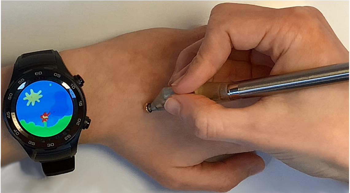
Figure 5.1: Suggested application scenario of the pen prototype PentelliZen: When the pen tip touches the skin, strokes can be drawn. A cursor on the display shows the corresponding position of the pen. To maximize visibility, menus are hidden at the edge of the display. The size of the drawing area, color, and size of the strokes can be adjusted via mid-air interaction with spatial menus.
