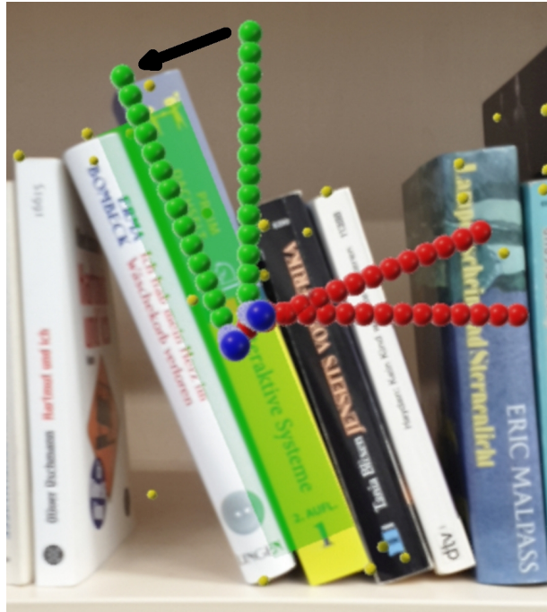
Figure 8.4: Debug view of a highlighted book with displayed AR feature points: Angular differences are also taken into account. There are minor deviations from the center point caused by the movement of the camera and the resulting deviation of the anchor points.
