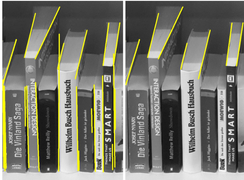
Figure 8.3: Line rejection: Initially extracted lines (left) and lines to be rejected (right). The lower endpoints of the rejected vertical lines are subsequently used to create the bounding boxes.
