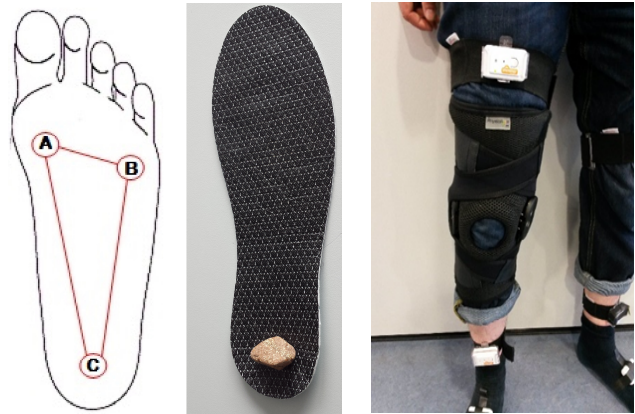
Figure 3.10: Knee brace and modification of the support point of the foot. Support points: (A) Caput des Os metatarsae I, (B) Caput des Os metatarsae V and (C) Tuber calcanei
