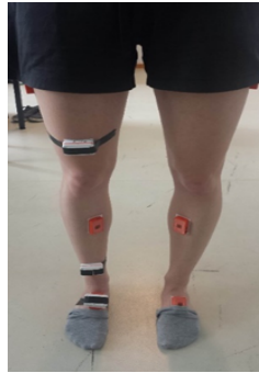
Figure 4.9: Shimmer (white) and reference (orange) sensor system platform.
