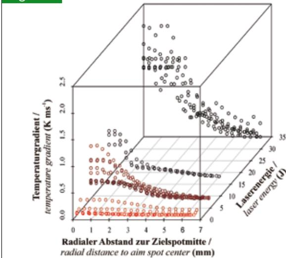
Influence of applied laser energy (Gauß-beam with ø 6 mm) on temperature gradient relative to the aim spot center
