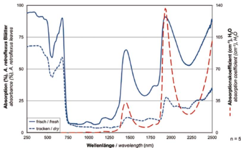
Absorption spectra of fresh and dried leaves (*A. retroflexus*) and the absorption coefficients of water
