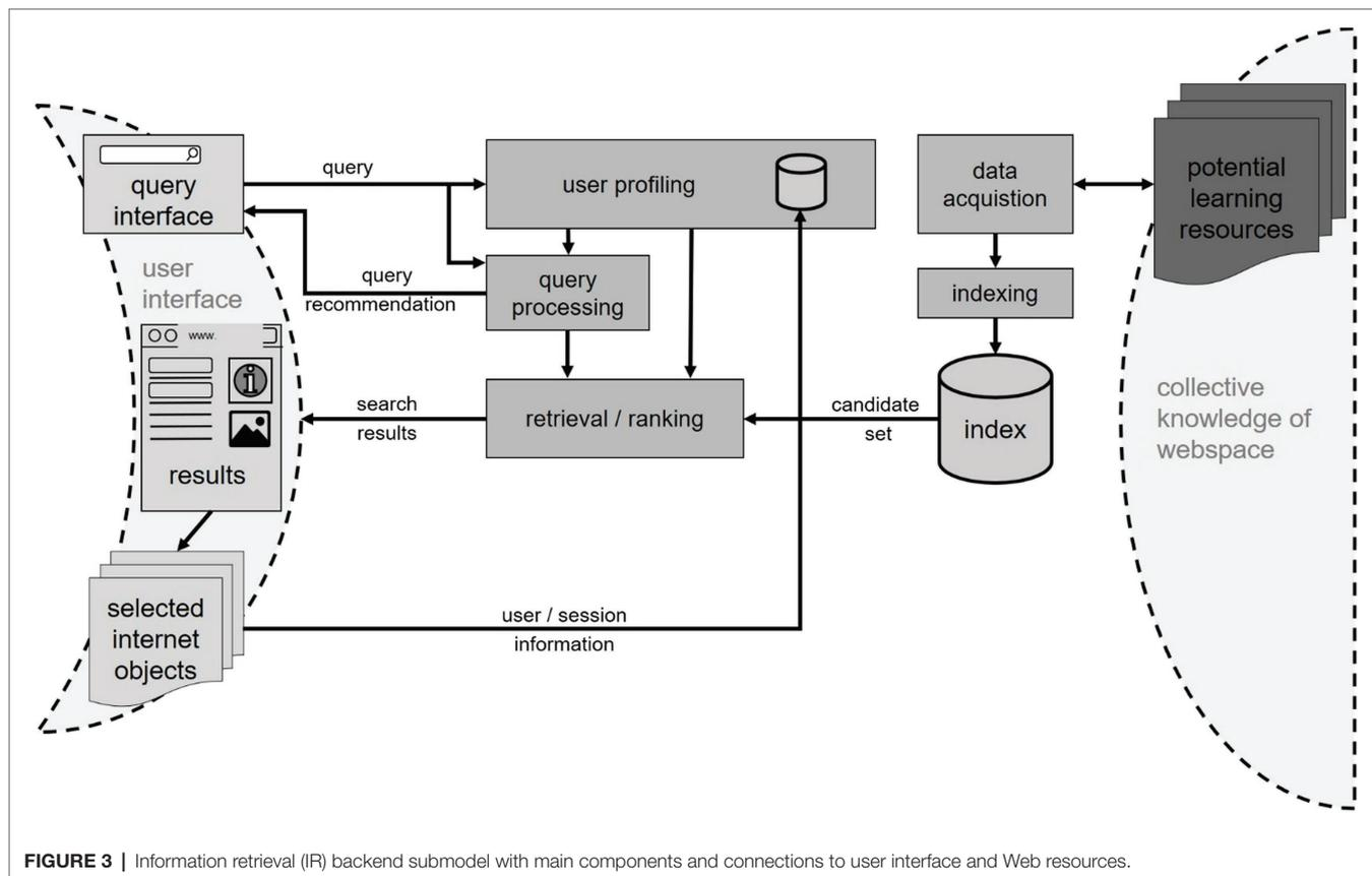
**FIGURE 3 |** Information retrieval (IR) backend submodel with main components and connections to user interface and Web resources.
