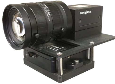
Figure 8.2: Image of the multi-sensor system consisting of a camera and an IMU.
