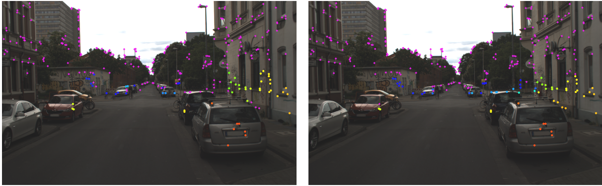
(a) Stochastic features colored by depth (red: close, blue: distant, violet: no depth). (b) Interval features colored by depth midpoint (red: close, blue: distant, violet: no depth).
