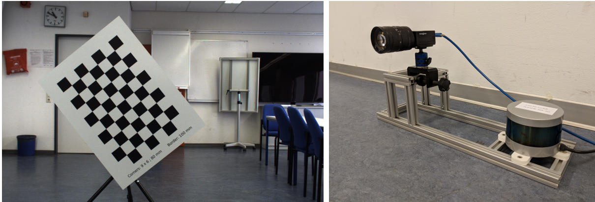
(a) Exemplary calibration image which depicts the calibration environment as well as the employed checkerboard. (b) Multi-sensor system, consisting of a camera and a laser scanner, that is employed to evaluate the extrinsic calibration.
