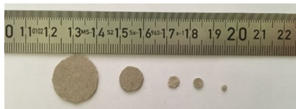
Figure 1. Flaw imitations with a diameter of 20, 10, 5, 4, and 2 mm, from left to right, with a thickness of 0.6 mm.
