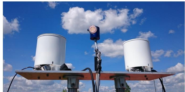
Figure 4. Photo of the measurement devices mounted on the measurement platform. Left: UV-BTS, centre: entrance optic of the NDACC device, right: VIS-BTS.
