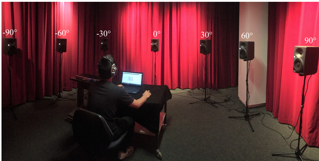
Figure 7. A photograph of the experimental setup. Seven loudspeakers were positioned at -90^\circ , -60^\circ , -30^\circ , 0^\circ , 30^\circ , 60^\circ , and 90^\circ relative to the subject with a distance of 1.9 m. The subject evaluated the externalization ratings of test stimuli via a graphical user interface (GUI) implemented on the Max/MSP platform [31] on a Thinkpad laptop. The Fireface UFX+ audio interface can be seen on the left side of the laptop.
