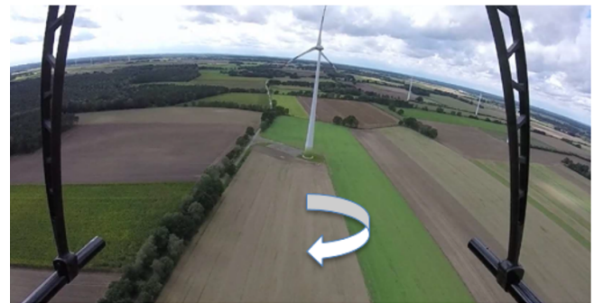
Figure 13. Picture taken from a video stream during hover flight. The camera is facing towards the CVOR in 3 km distance. Later the UAS rotated around its vertical axis clockwise during measurement (cp. Measurement data in Fig. 12).
