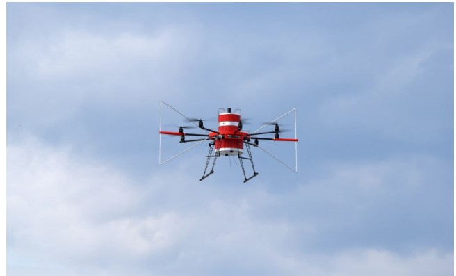
Figure 1. The UAS (octocopter PTBee 3) with a bow-tie antenna for VHF measurements. Its centre of gravity matches the phase centre of the antenna which results in a dipole-like reception pattern.
