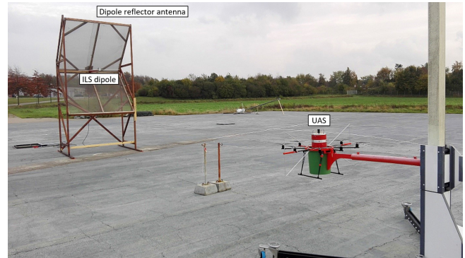
Figure 7. UAS measurements of the electrical field strength in front of the dipole reflector antenna (DRA).
