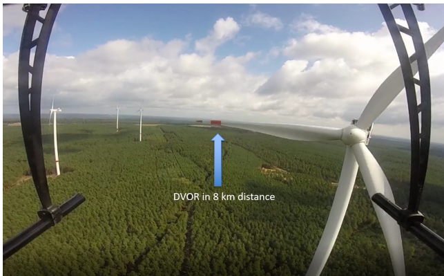
Figure 11. Picture from the video stream taken during a hover flight at hub height behind a wind turbine. The camera points towards the DVOR in about 8 km distance. In this position the data from Fig. 10 was measured.
