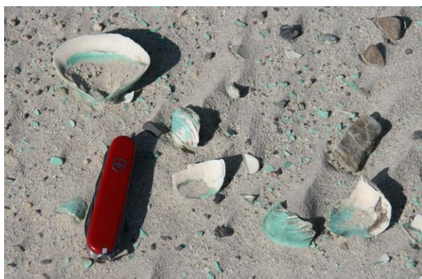
Figure 5. Secondary copper minerals on the surface of the tailings dump at Chañaral Bay and on the marine shells (Picture from BGR).
