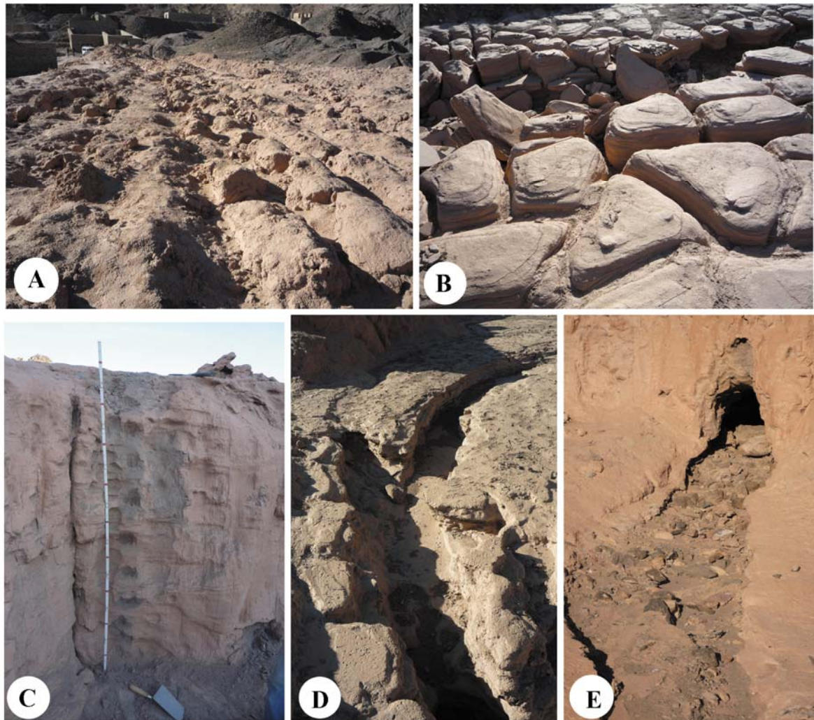
Fig. 2.5. Barramiya gold mine tailings: (A) Surface view, locally with wide desiccation cracks with partly intensive erosion (B); the position of the profile (C); erosion effects at deep desiccation cracks (D); and subrosion channels at the bottom (E) of the tailings caused by intensive flooding.
