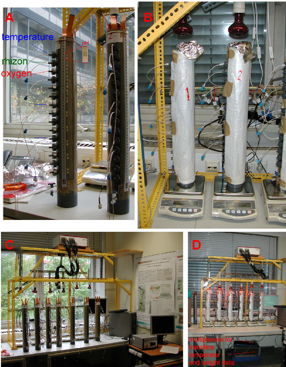
Fig. 4.5. Showing the distribution of the sensors along the column (A), Isofelt used to prevent heat loss/ infiltration from the sides of the column, and the measurement environment around the columns (B-C).
