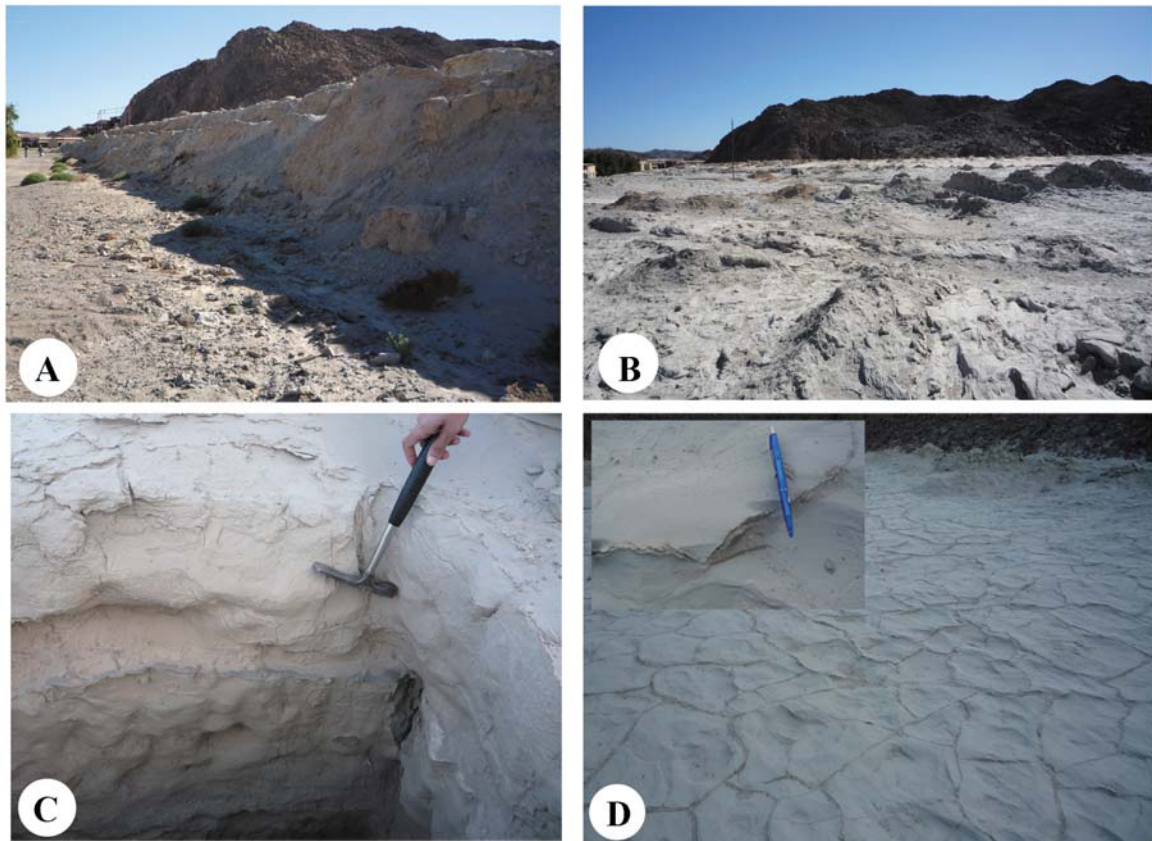
Fig. 2.3. El Sid gold mine tailings: Lateral (A) and surface (B) views of the profile position with a thin hardpan of gypsum (C) and gypsum crystallization on both sides of sediment refilled desiccation cracks, and close to the crack in patchy distribution (D) narrow desiccation cracks and polygons at the surface of the tailings.
