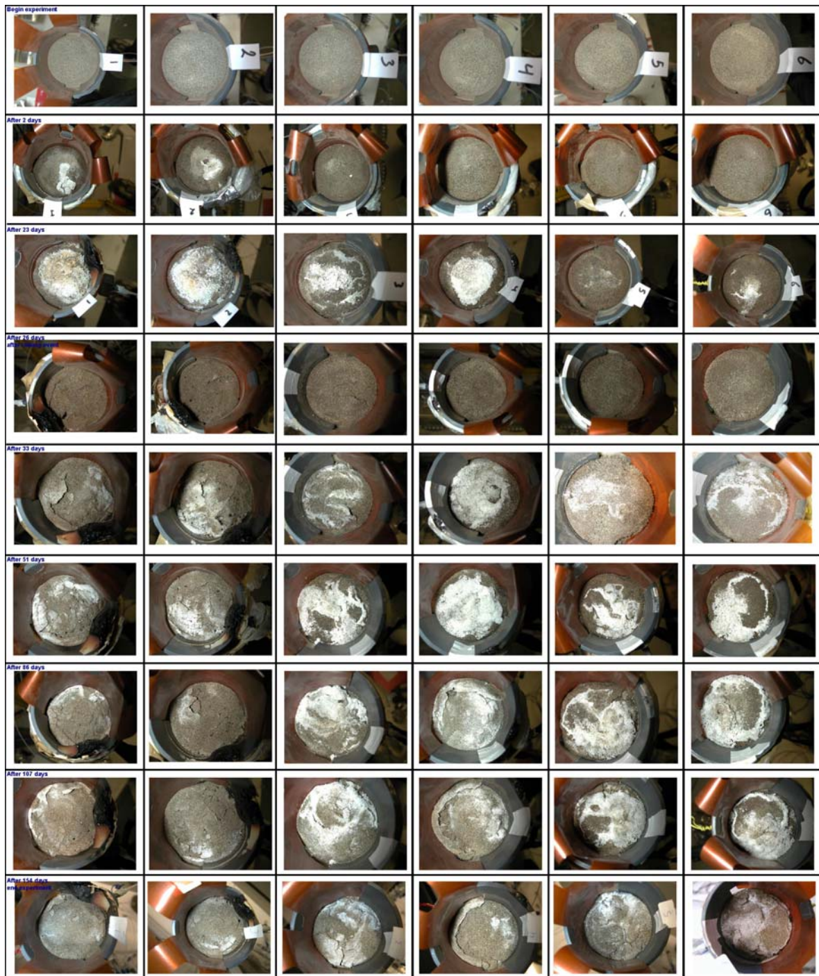
Fig. 4.18. Time series of efflorescence on column tops.
