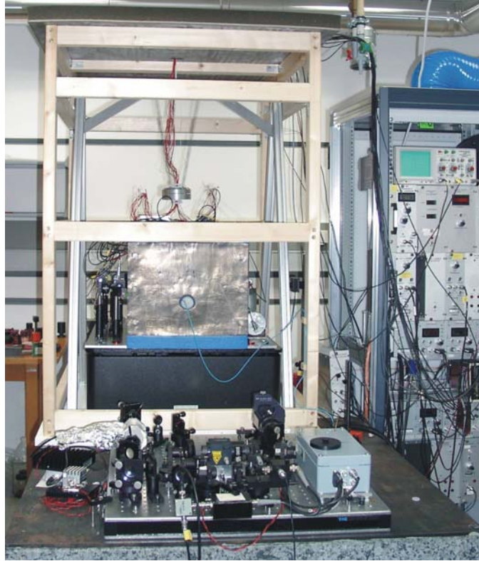
Fig. 3.15 Vibration isolation system. The reference cavity is within the lead covered styrofoam box, which is situated on the top of the vibration isolation platform (Minus-k). The setup is surrounded by an additional acoustic isolation box (not yet installed on the photo).
