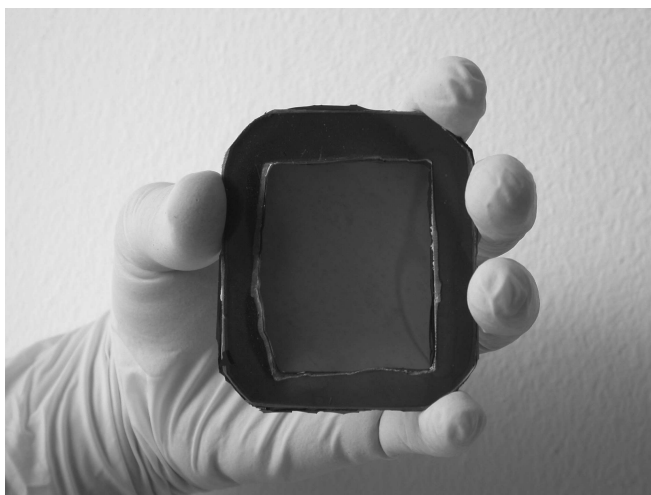
Figure 3.6. Photograph of a \sim 25\ \mu\text{m} thick free standing SPS thin-film. A plastic frame mechanically stabilises the sample. The dissolving of a highly porous separation layer during sintering permits the separation of the porous film from the silicon substrate.
