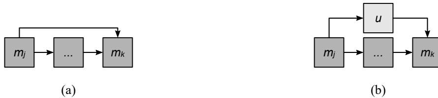
Figure 8: Bypassing structure (a) and the transformation to a parallel structure (b) by adding a virtual unit u .
