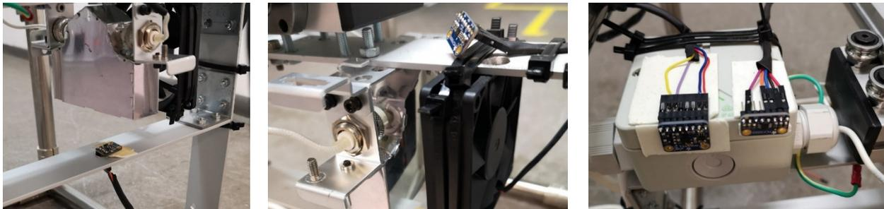
Figure 3: UV sensor under the UV lamp with reflector unit, temperature sensor next to the UV lamp, acceleration and temperature sensor in the upper part of the printing chamber (from left to right)
