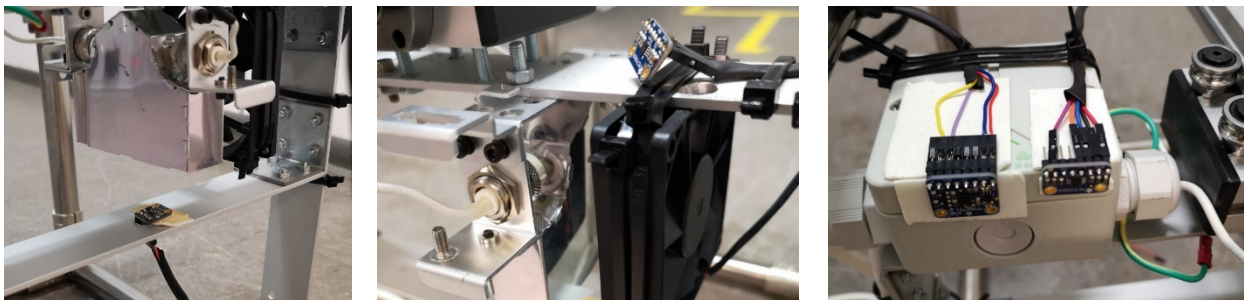
Figure 3: UV sensor under the UV lamp with reflector unit, temperature sensor next to the UV lamp, acceleration and temperature sensor in the upper part of the printing chamber (from left to right)
