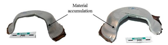
Fig. 5. Pictures of deep drawn sandwich cups. Left: 1.2 mm thick GRP. Right: 2.5 mm thick GRP.
