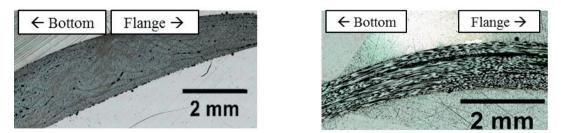
Fig. 6. Micrographs of GRP in the side wall axial (left) and at the punch edge perpendicular (right) to the fibre direction.
