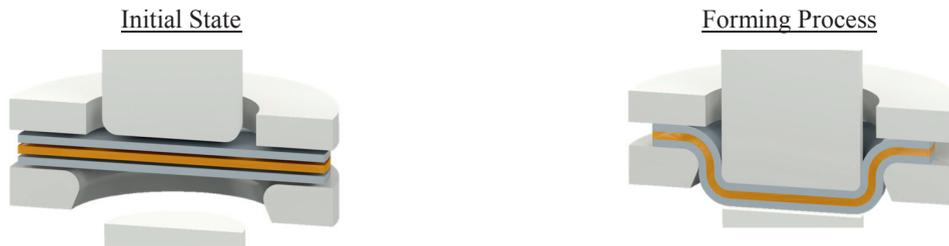
Fig. 3. Schematic illustration of the deep drawing process using non-joined metal-FRP-sandwiches.
