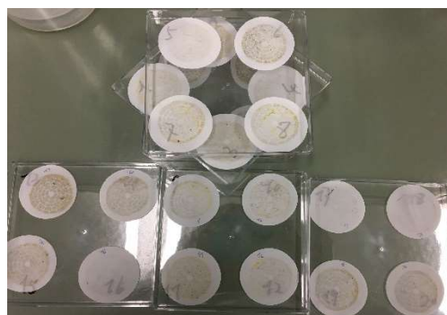
Photo B.2 The after dried nylon hydrophilic membrane filter with particulate matters
