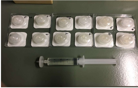
Photo B.3 Samples of chloroform solution for filtration by filter unit with PTFE membrane filter (pore diameter 0.2 \mu m)
