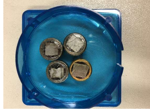
Photo B.4 Samples leaf surface which was covered by carbon for SEM scanning
