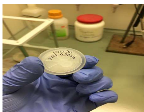
Photo A.9 PTFE membrane filter with pore diameter of 0.2 µm to filtrate chloroform solution
