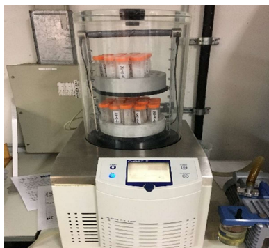
Photo A.1 Vacuum Freeze Drier (Alpha 1-2 LD plus Entry Freeze Dryer package, Martin Christ, Australia)
