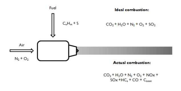
Figure 5.1 Scheme of the jet fuel combustion (Timmis 2015)
