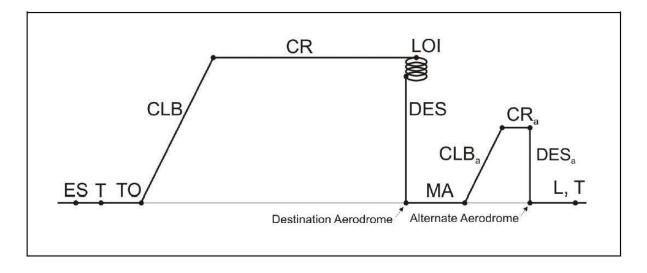
Figure 3.5 Typical profile of a civil mission (Scholz 2019b)
