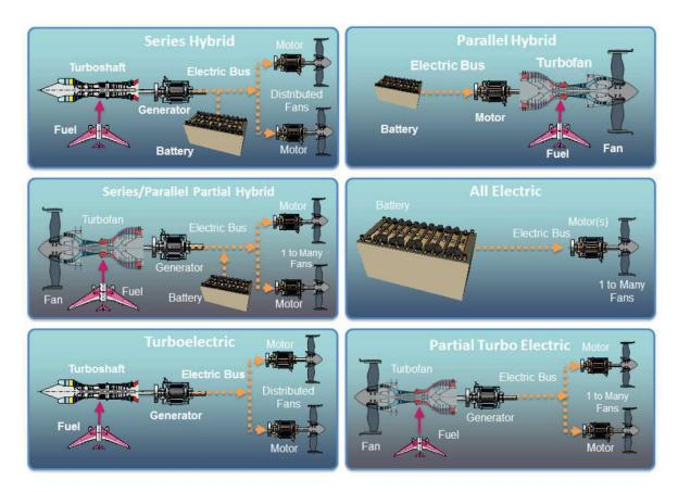
Figure 2.1 Types of electric propulsion (NAP 2016)
