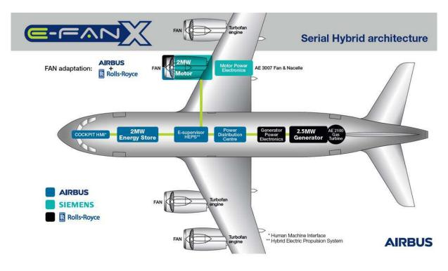
Figure 3.1 Internal configuration of the E-FAN X (Bjorn 2017)
