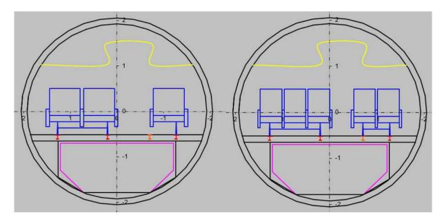
Figure 3.8 Cross section for the BAe 146-100 and E-FAN X by AERO (2011)
