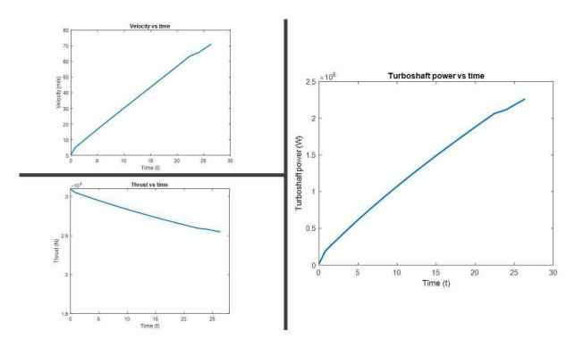
Figure 3.2 Values of velocity, thrust and power for a sea level take off
