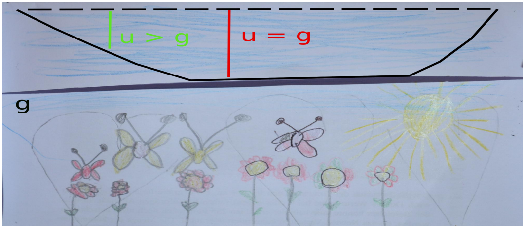
Figure 61: Obstacle problem -u'' = -1 in \Omega and u(0) = u(1) = 0 : deformation u of a line that is constraint by the obstacle g .
