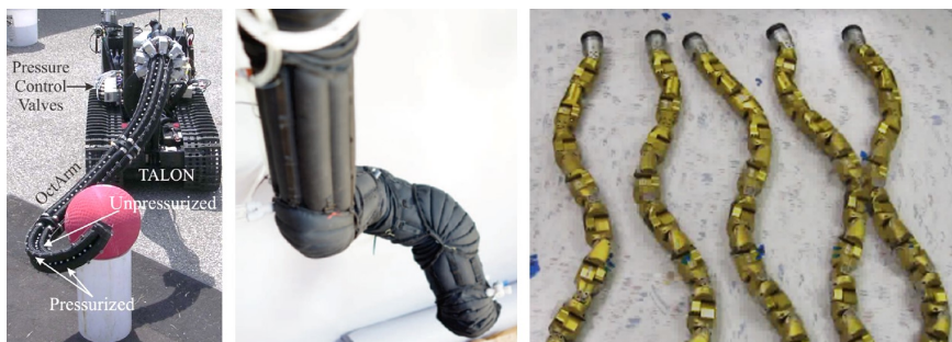
Figure 14: OctArm (left) (reprinted from (Trivedi, Dienno, and Rahn, 2008), © 2008, with kind permission from ASME), a soft pneumatic robot (middle) (reprinted from (Bodily, Allen, and Killpack, 2017), © 2017 IEEE), and snake robots (right) (reprinted from (Tesch, Schneider, and Choset, 2013), © 2013 IEEE).
