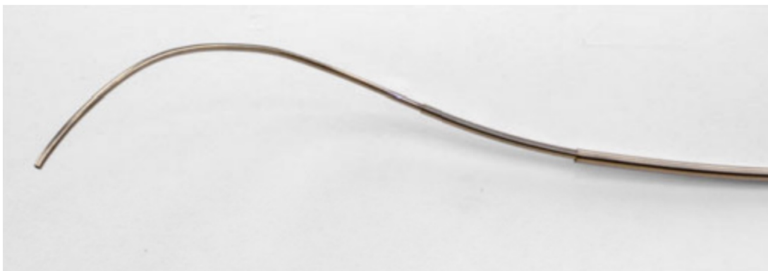
Figure 1: Concentric tube continuum robot composed out of three tubes (reprinted from (Gilbert, Neimat, and Webster III, 2015), © 2015 IEEE)
