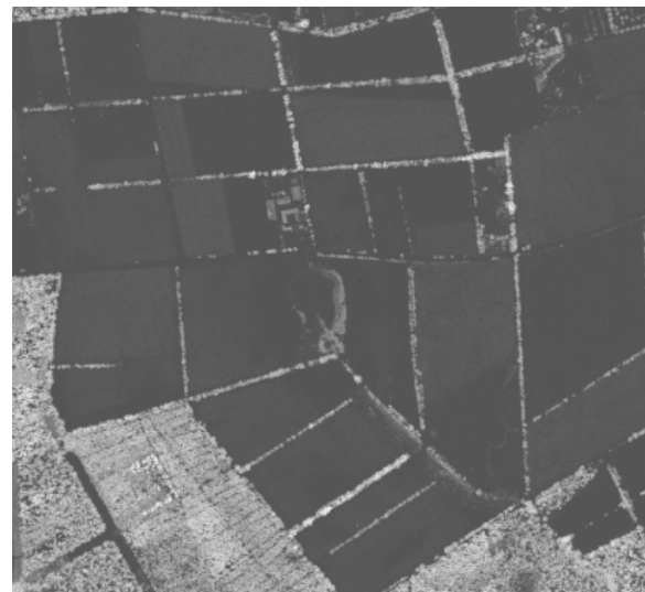
Figure 3. Example data from the LIDAR acquisition. This scene represents the same temporal and spatial location as depicted in Figure 2. Higher structures (mainly vegetation but also some houses) have lighter shades of grey.
