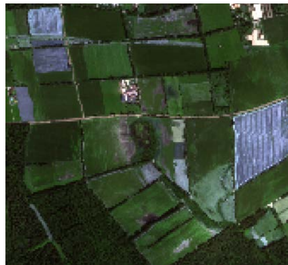
Figure 5. Simulated RGB data set representing the Sentinel-2 bands 2 to 4. The scene is spatially and temporally identical to Figures 2 and 3. The spatial resolution here is 10m.
