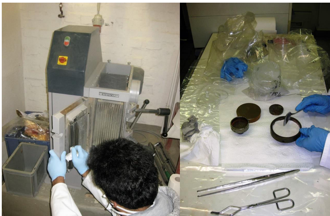
Fig.3.2. Crusher unit (left) and packing of the milled samples into petri dishes (right)
