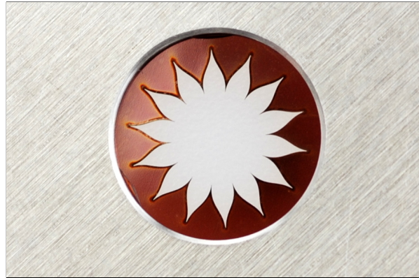
Figure 4.20: Photograph of the apodized aperture in aluminum mount. The bore in the aluminum mount has a diameter of 8 mm. This aperture is used for the flat-top generator of the TS as explained in Section 4.3.4.
