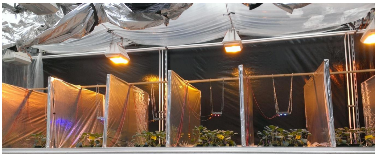
Fig. 3 Greenhouse chamber separated in different independent light compartments equipped with sodium vapor lamps and additional specific high-power LED-panels with UV-B, UV-A, blue, or red wavelengths for Brussels sprout plant illumination.
