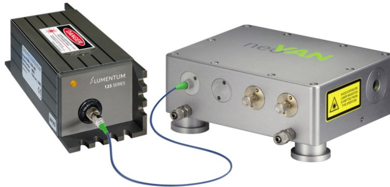
Fig. 4.14 Picture of the Lumentum NPRO 125N-1064. It is connected by a single mode fiber to a neoVAN amplifier.
