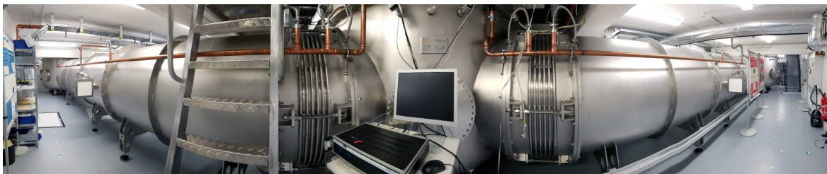
Fig. 3.1 The AEI 10 m Prototype facility with 100 \text{ m}^3 volume, 3 m diameter tanks and 1.5 m diameter beam tubes. The ultra-high vacuum system is designed in a rather generous way, such that it can hold more than one experiment at a time. The pressure inside the system is below 10^{-6} mbar after 12 hours of pumping, after one week it is below 10^{-7} mbar.
