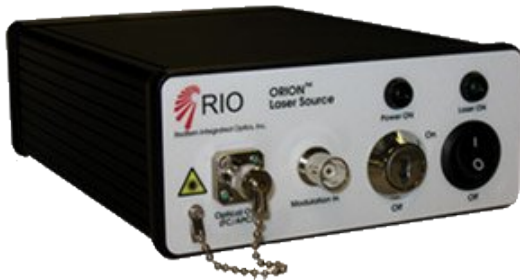
Fig. 4.10 Image of an OEM version of the 20 mW RIO ECDL. It has a wavelength of 1064 nm. The diode is coupled to a FC/APC fiber.
