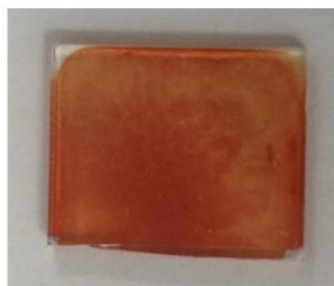
Figure SI-7. Photograph of the film (size approximately 1 cm) prepared by drying MUA-CdSe/CdS (aq) solution on a glass slide under ambient conditions. The optical density (of the absorption measured in an integrating sphere) is 1.1 at 300 nm wavelength.
