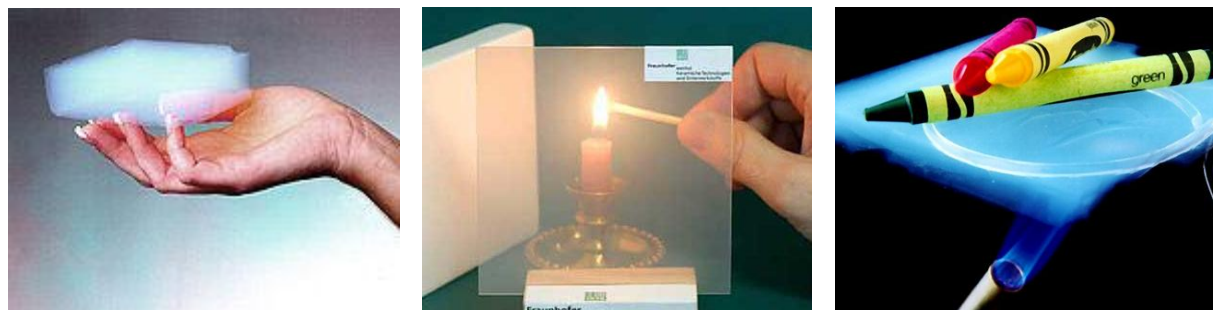
Figure 14. Photographs of silica aerogels showing its physical properties such as i) extremely light weight, ii) optically transparent in nature iii) low thermal conductivity. Photographs are reprinted with permission from Wiley and Nature publishing group.
