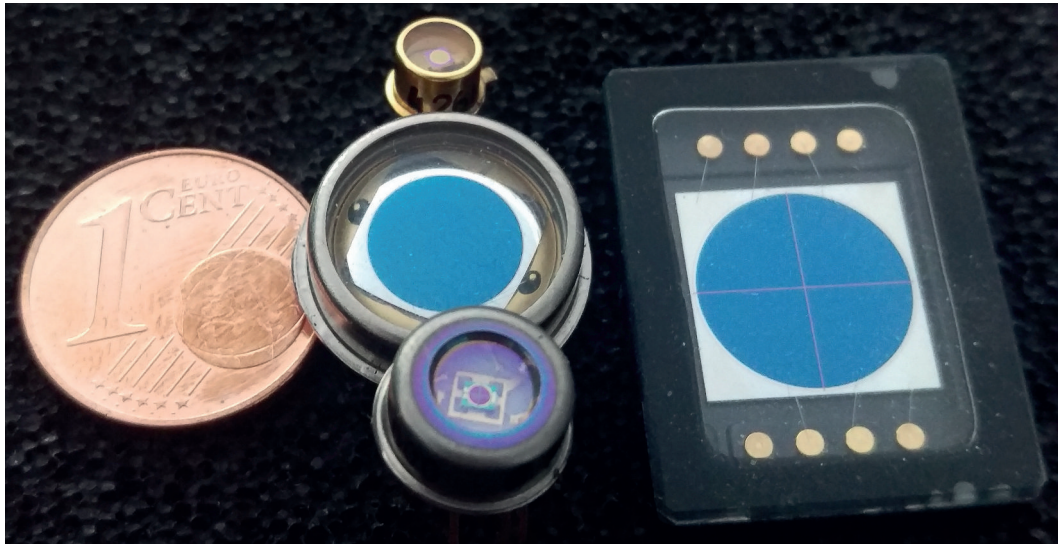
Figure 2.10: Photograph of a large circular single-element photodiode (center), a small quadrant-photodiode with barely visible gaps (bottom), and a large quadrant photodiode (right).
