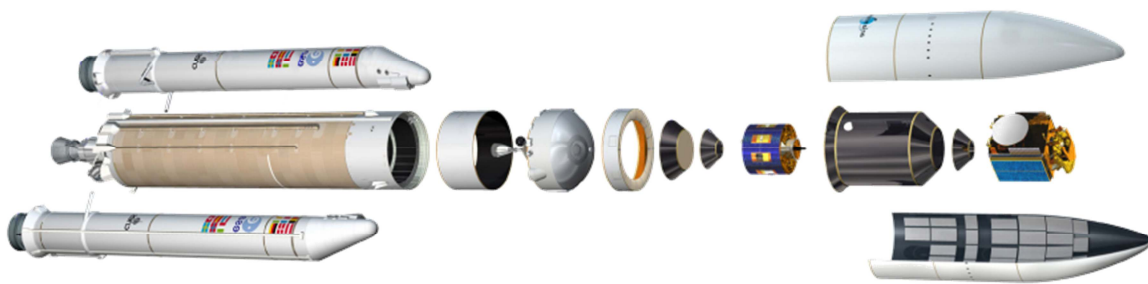
Figure 1-1: Exploded view of Ariane 5 ECA, compare [1]
