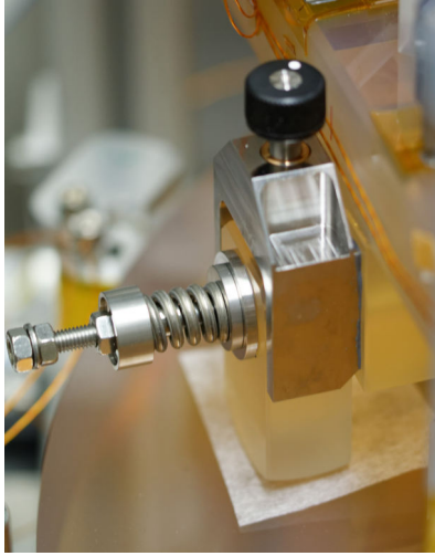
Figure 3.6: One of the adjustable feet for the tip-tilt mount to align the telescope simulator baseplate. The upper Zerodur ® block is bonded to the underside of the telescope simulator and clamped together with the lower Zerodur ® block with a spring loaded screw. For adjusting the height of the foot the fine pitch screw in the metal bracket on top of the lower block pushes on the lower block and the two Zerodur ® parts slide against each other when the spring loaded screw is loosened.
