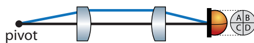
Figure 2.10: Removing beam walk on the photodiode with an imaging system. The pivot is imaged on the center of the photodiode surface.
