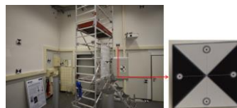
Figure 2. Calibration room (left) depiction of detected centroid of circles using sub-pixel target mode of the PhotoModeler software (right)
