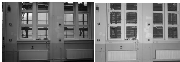
Figure 4. Rectified image (left), Reflectance image from TLS (right)
