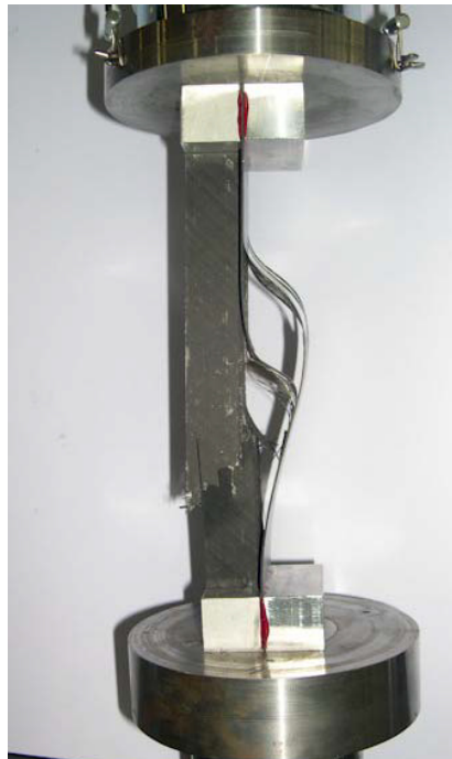
Figure 1.2: Collapse of a composite laminate due to the delamination (Bisagni, 2006).
