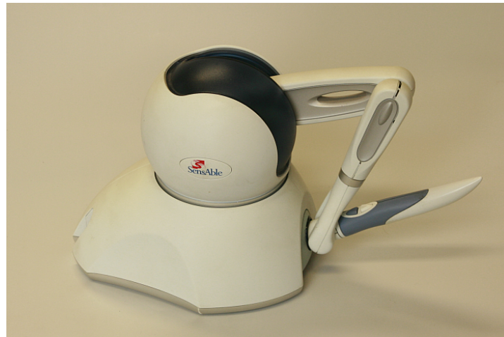
Figure 4.14: Phantom Omni haptic device
