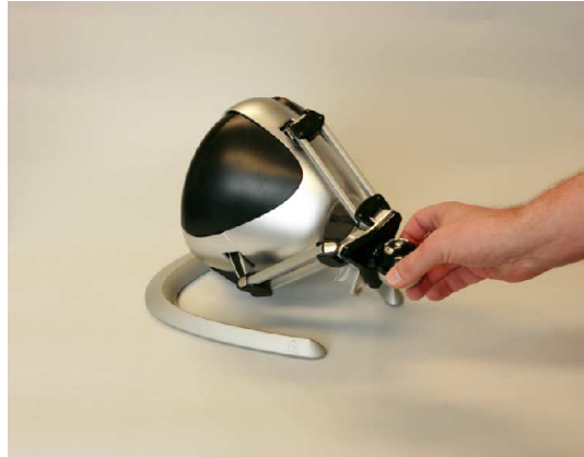
Figure 2.6: Example of a 3-DoFs haptic display: Novint Falcon
