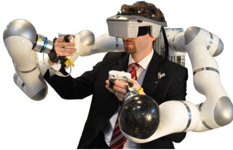
Figure 3.17: The DLR’s bi-manual haptic interface used in the VR simulator for telerobotic on-orbit servicing (source: [200])
