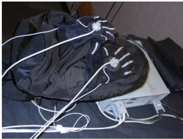
Figure 2.4: Limb tracking device ( Polhemus FastTrak ) (source: [100])
