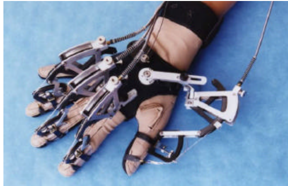
Figure 2.8: Example of an n -DoFs device (source: [14])
