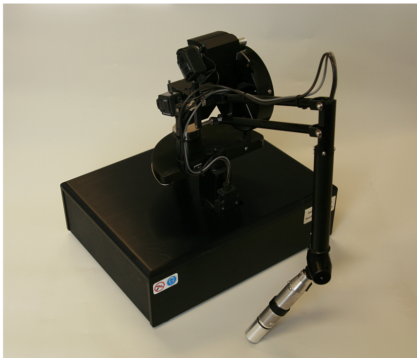
Figure 4.15: Phantom Premium 1.5 6-DOF haptic device
