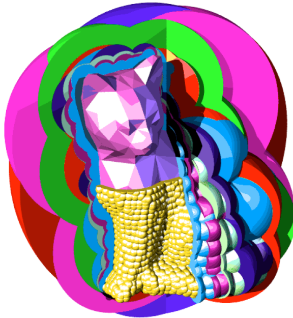
Figure 3.15: Cut of the bounding spheres hierarchy (source: [198])
