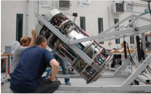
(a) The capsule being rotated around a horizontal axis using a hydraulic crane.
