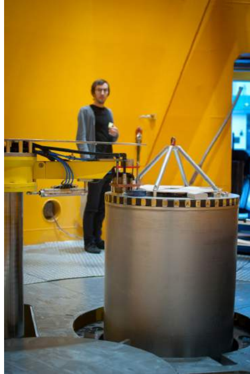
Figure 37: The capsule sits in the catapult receptacle and is docked with the supply arm prior to evacuation of the tower. Once the setup is retracted to launch position 9 m below the drop tube, the scientist have a 5 min launch window before the process is aborted.
