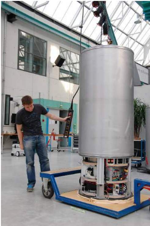
Figure 32: Capsule hull is lowered onto the capsule for the first pre-test. The two visible platforms at the bottom constitute the capsule base structure. The lowest level holds most of the systems batteries. The next platform houses the secondary capsule control computer in charge of communication to the control room.
